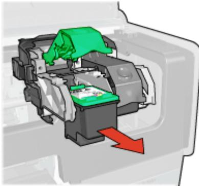
6. Remove the replacement print cartridge from its packaging and carefully remove the plastic tape. Hold the print cartridge so that the copper strips are on the bottom and facing toward the printer.
