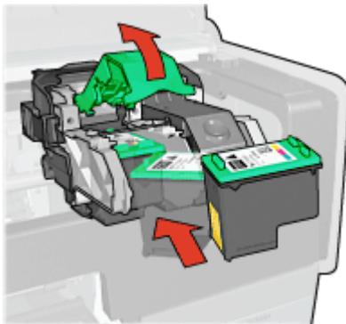
8. Push down on the print cartridge latch until it snaps closed.
