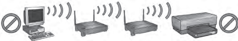
1 | The computer and the printer are on different subnets.
