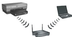
Use this connection type if you want a wireless (802.11b or g) connection between the printer and your network.
