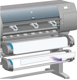
6. Rotate the spindle backwards to move the paper edge out of the way.
