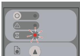
This indicates that the scanner needs to make some readjustment but is unable to do so. Remove all paper from the scanner, ensure the insertion slot height is set to minimum, and wait for the light to turn off.
