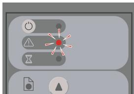
The most likely explanation is that the scanning area needs cleaning. Perform the routine maintenance procedures explained in your online guide, which include cleaning. Restart the scanner when you have finished the maintenance procedures.
