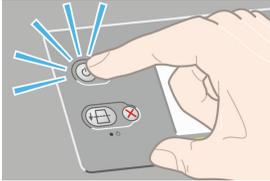
When you switch off the printer this way, the printheads are automatically stored with the printhead cleaners, which prevents them from drying out.
