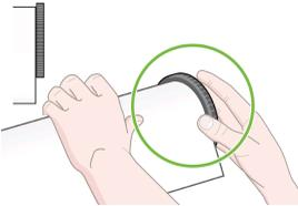
7. Put the blue paper stop on to the other end of the spindle, and push it towards the end of the roll.
