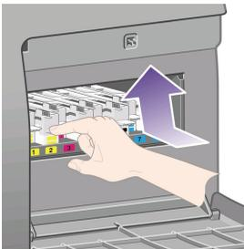
4. Lift up the printhead cleaner to remove it from the slot, and slide it out horizontally as shown below.
