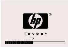
If the printer's start-up process stops when the front panel is displaying the number 17, this indicates that there is a problem with the file system on the printer's hard disk, so the printer is checking the whole file system and making any necessary corrections. This problem can arise when there has been a power cut while the printer was switched on, or if there is a physical problem with the hard disk.
