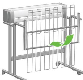
2. Remove the pin from each leg extension, and rotate the leg extension upwards.
