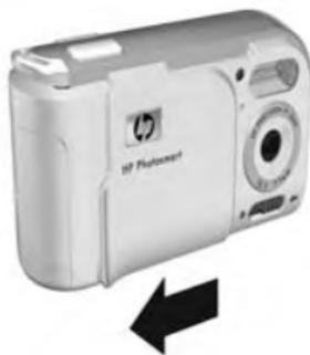
To turn the camera off, slide the lens cover closed until it clicks, covering the lens.
