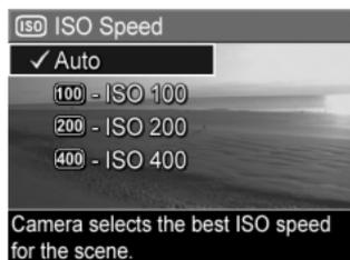
If the setting is anything other than the default **Auto** setting, the icon for the setting (as shown in the **ISO Speed** sub-menu) will appear in the **Live View** screen. The new setting remains in effect until it is changed again or until the camera is turned off. The **ISO Speed** setting resets to the default **Auto** setting when you turn the camera off.
