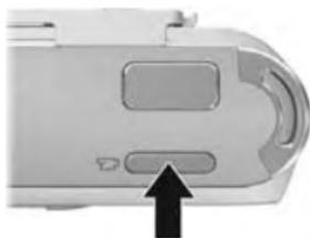
After recording has stopped, the first frame of the video clip appears for three seconds on the Image Display. This is called **Instant Review**. You can delete the video clip during **Instant Review** by pressing the
