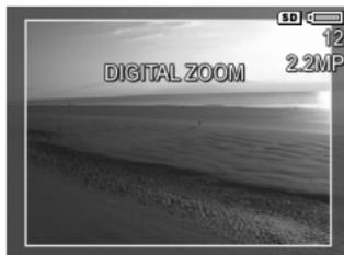
The resolution number on the right side of the screen also becomes smaller as you digitally zoom. For example, **2.2MP** appears in place of **5MP**, indicating that the image is being captured at a size of 2.2 Megapixels.
