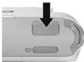
2. Press the **Shutter** button to take the picture. The camera beeps after taking the picture.
