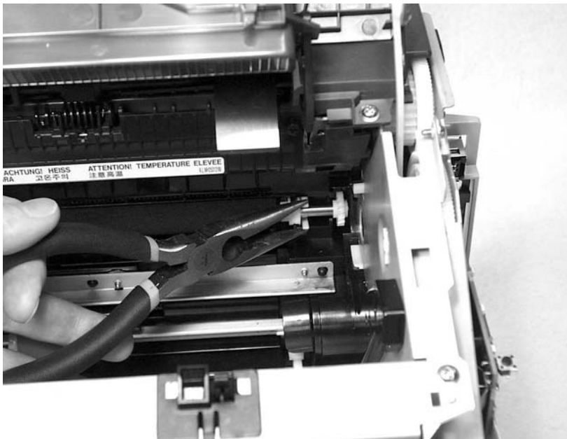
Figure 5-22 Remove the transfer roller (3 of 3)
