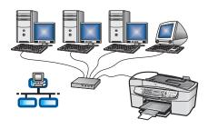
Use this connection type if you want an Ethernet cable connection between the device and your network.
