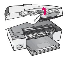
Lift the print cartridge door until it stops. The print carriage moves to the right.
