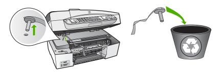
After you remove the orange shipping lock, turn off the HP All-in-One, and then turn it on again.
