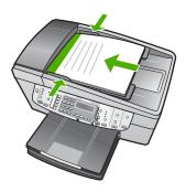
Tip For more help on loading originals in the automatic document feeder, refer to the diagram engraved in the document feeder tray.
