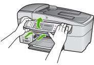
Retain the control panel faceplate. Do not return the control panel faceplate with the HP Allin-One.
