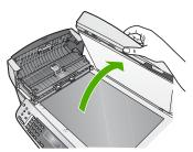
4. Lift the automatic document feeder mechanism.
