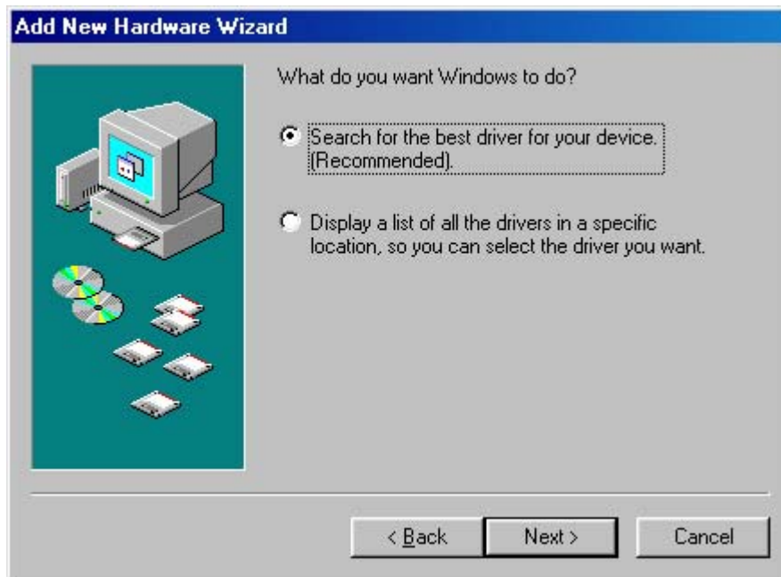
Figure 4-3 Add New Hardware Wizard USB Composite Device - Search for driver dialog box
