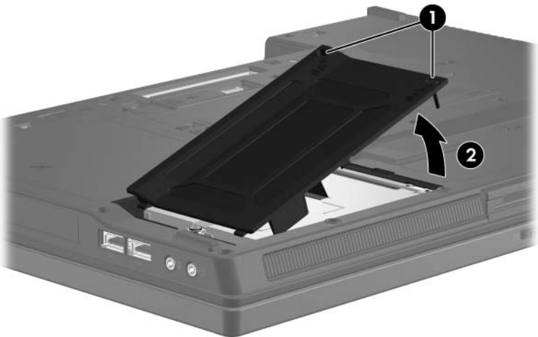
Removing the Hard Drive Cover
