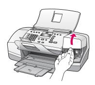
Lift the print cartridge door. The print carriage moves to the right side.
