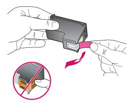
Pull the tab to remove the tape from **both** print cartridges.
