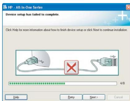
**Problem:** (Windows only) The **Device Setup Has Failed To Complete** screen displays.
