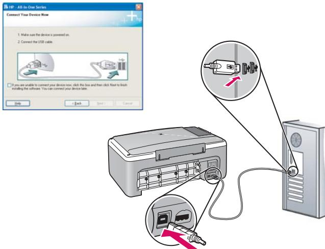
**EN** **Windows:** Once the USB prompt appears, connect the USB cable to the port on the back of the HP All-in-One, and then to any USB port on the computer.
