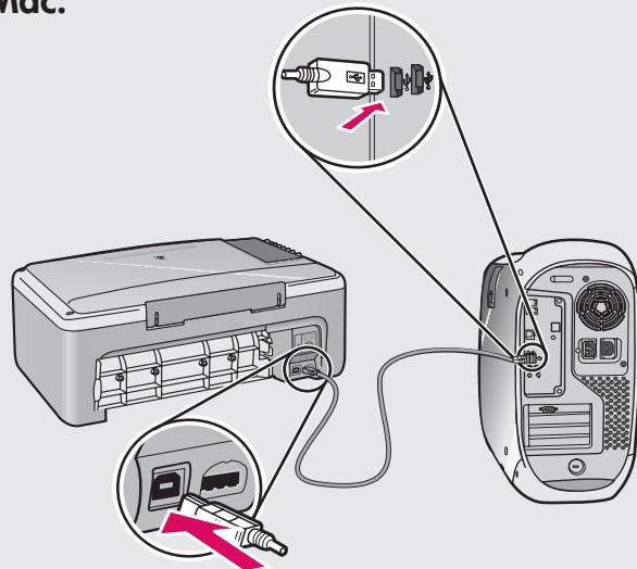
**EN** **Mac:** Connect the USB cable to the port on the back of the HP All-in-One, and then to any USB port on the computer.
