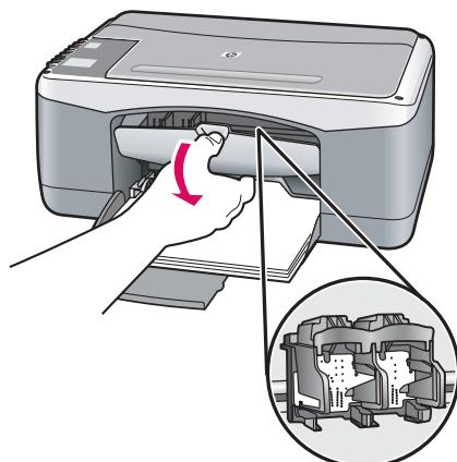
**EN** Open the print cartridge door. Make sure the print carriage moves to the center.
