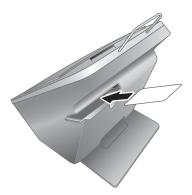
To scan a card using the card slot on the back of the printer, follow these steps:
