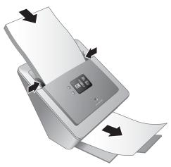
3. Adjust the paper guides to center the original. Make sure the paper guides touch the edges of the original.
