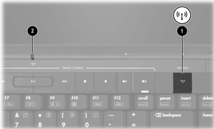
You can enable and disable the wireless devices with the wireless button. You can also enable and disable the wireless devices in the Setup Utility.
