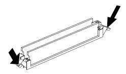
**8** Hold the memory module by its edges only, as you lift it away from the socket. Store it in its antistatic packaging.
