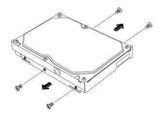
**NOTE:** If your hard disk drive does not include the screws, you may need to purchase four additional screws. If your hard disk drive screws are torx screws, you may need a torx screwdriver.
