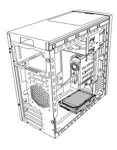
5 Attach the data and power supply cables to the back of the hard disk drive.
