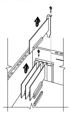
**5** Loosen the screw on the card you are replacing. Hold the card at the top and carefully pull the card straight out of the add-in card slot.
