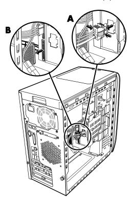
**5** Disconnect the power cable and data cable from the back of the hard disk drive (B). For a Serial ATA drive, press the latch (1) (select models only) in the center of each plug and pull the plug (2) from the drive connector. For a Parallel ATA drive, use a gentle rocking motion to free the plug.
