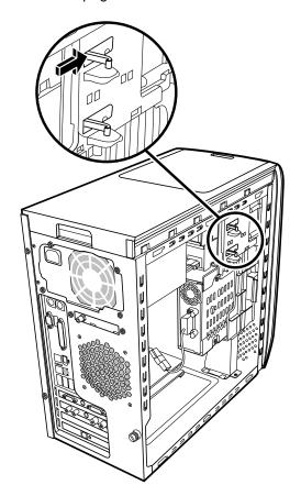
**3** Lift the plastic tabs on the side of the optical drive you want to remove. Push the drive part way out through the front of the PC.
