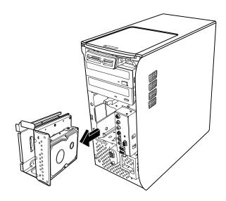
8 Gently lay the drive bay flat with the hard disk drive on top.
