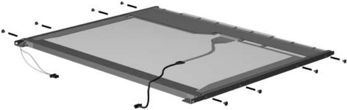
Removing the LCD Panel Frame Screws
