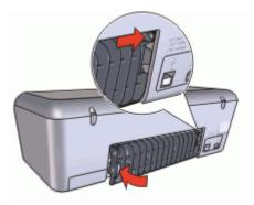
6. If the paper jam cannot be removed from the back of the printer, raise the printer cover, remove the paper jam from the front of the printer, and then lower the cover.
