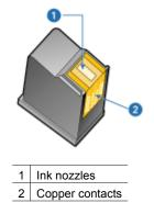
6. Slide the print cartridge firmly into the cradle at a slight upward angle until you feel resistance.
