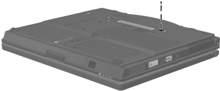
Torx8 T8M2.0x5.0 Screw Location
