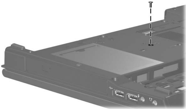
Torx8 T8M2.5x4.0 Screw Location
