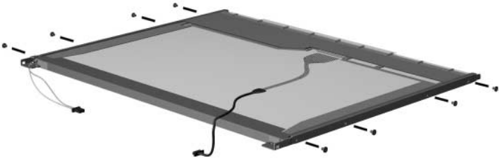
Removing the Display Panel Frame Screws
