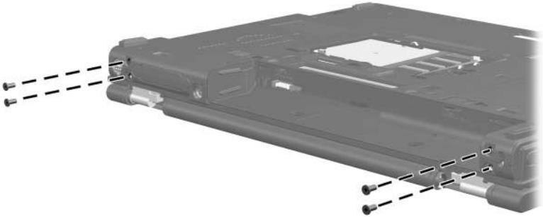
*Removing the Display Assembly Screws*
