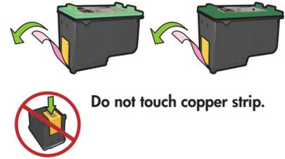
**6** Insert print cartridges. Push cartridges firmly until they 'click' into place.
