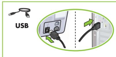
Make sure cable connections are secure.
