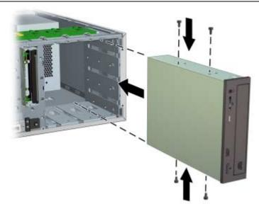
6. Slide the optical drive completely into a drive bay so that the drive is secured. On some workstation models, you will need to lift the spring-loaded latch on the left side of the optical drive cage while sliding the new drive in.
