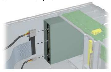
**NOTE:** Linux systems require the installation of the audio cable (see the illustration below). The location of the connector varies depending on your system. Refer to the documentation CD that shipped with your system for the appropriate location.
