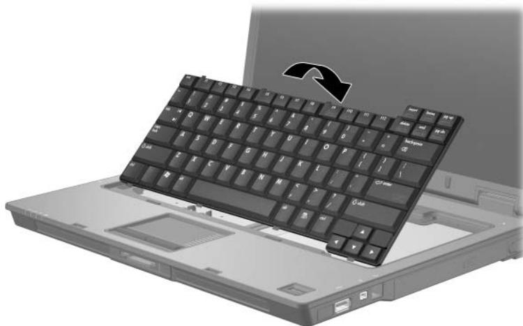
16. Slide the 4 keyboard latches to lock the keyboard.
