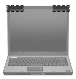
For optimal transmission, keep the areas immediately around the antennae free from obstructions.
