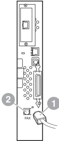
11. Connect the other end of the phone cord into the phone jack on the wall. Push the connector until you hear a click or until the connector is securely seated. Because there are different types of connectors, depending on the country/region, the connector might make an audible click when connected or might not make an audible click.
