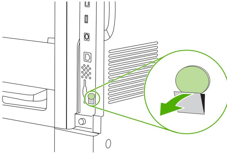
5. Open the formatter-cage door by grasping the metal tab and pulling the door open.
