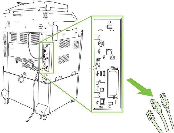
**NOTE:** If this is the first time the fax is installed, remove the small cover over the opening for the phone jack on the rear panel of the formatter before inserting the fax card into the formatter.
