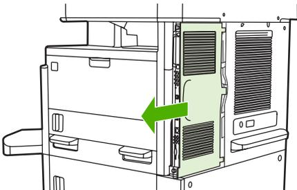
4. If necessary, remove the plastic fax-accessory cover from the formatter. Insert a coin into the groove at the top of the cover, and then pry the cover away from the formatter.
