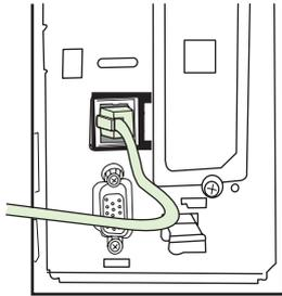
17. Connect the other end of the phone cord into the phone jack on the wall. Push the connector until you hear a click or until the connector is securely seated. Because there are different types of connectors, depending on the country/region, the connector might make an audible click when connected or might not make an audible click.
