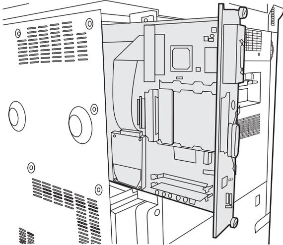
8. Reconnect any cables (4) removed from the formatter in step 4.
