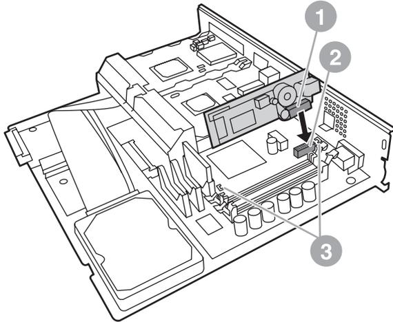
Install the formatter back into the MFP.
