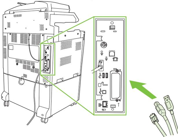
**NOTE:** When connecting the fax accessory to a phone line, ensure that the phone line being used for the fax accessory is a dedicated line that is not used by any other devices. Also, this line should be an analog line because the fax will not function correctly if it is connected to some digital PBX systems. If you are not sure whether you have an analog or digital phone line, contact your telecom provider.
