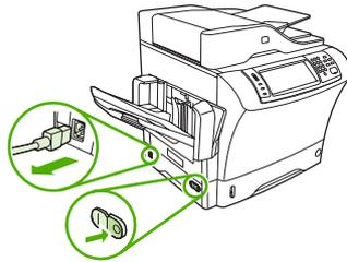
3. At the back of the device, remove the side cover by placing your fingers in the indented area and sliding the cover off.
