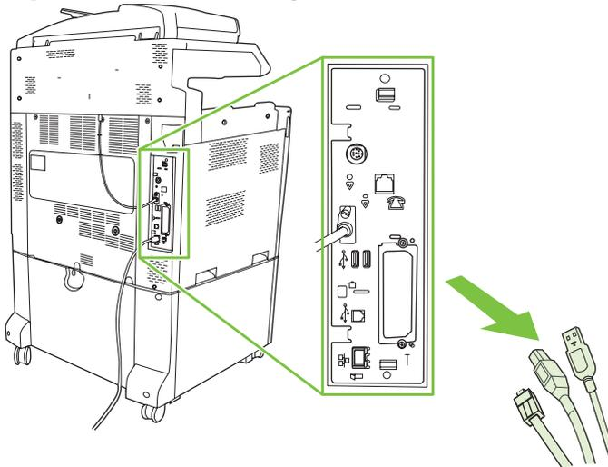
3. Pinch the black tabs at the top and bottom towards the center of the formatter board and then gently pull the board from the MFP. Place the formatter board on a clean, flat, grounded surface.
