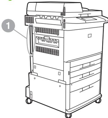
4. Disconnect all the cables (2) from the formatter (1). Remember where the cables are removed from to ensure that you reinstall them in the same locations.
