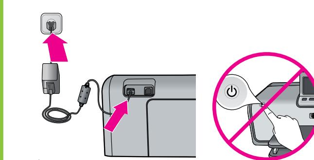
Wait until step 5 before turning on the printer.
