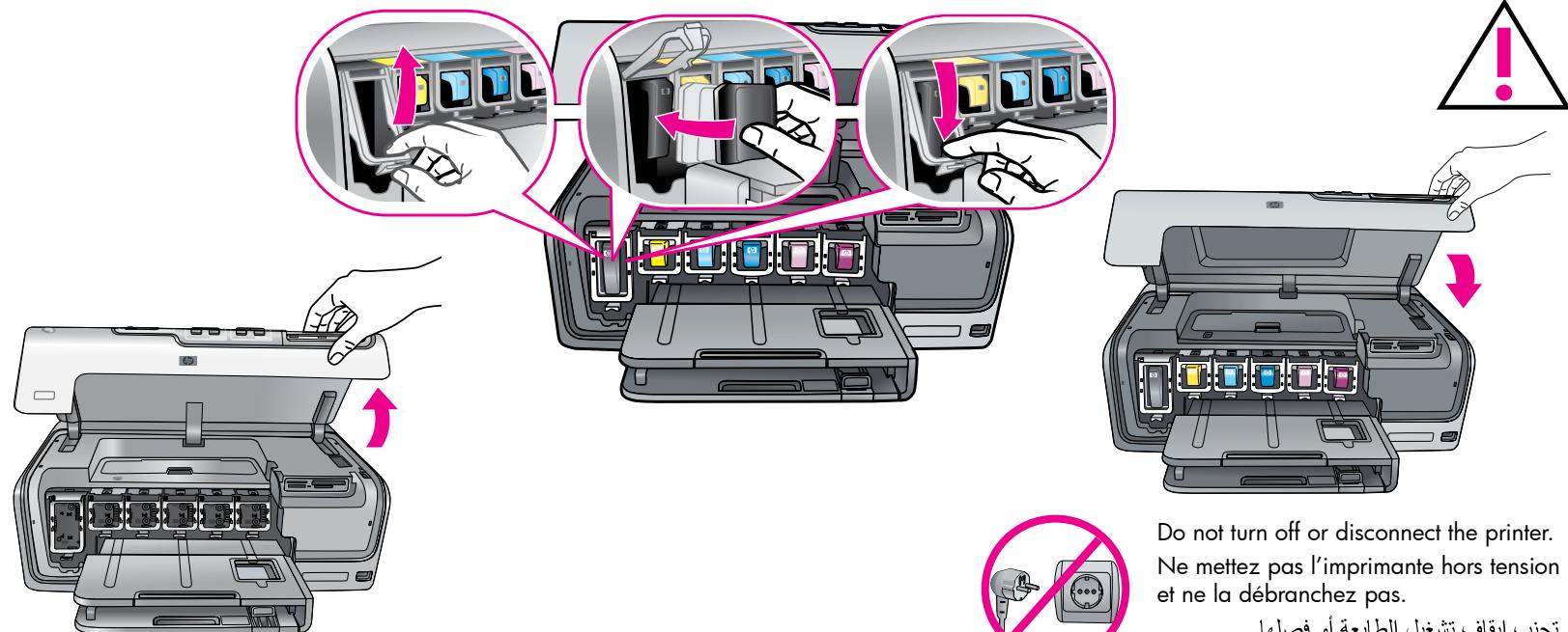
**Important!** A one-time initialization process begins after ink cartridge installation. Mechanical noises are normal and last about 4 minutes. Do not turn off or disconnect your printer. If the initialization is interrupted, see the troubleshooting section of the User Guide on CD.
