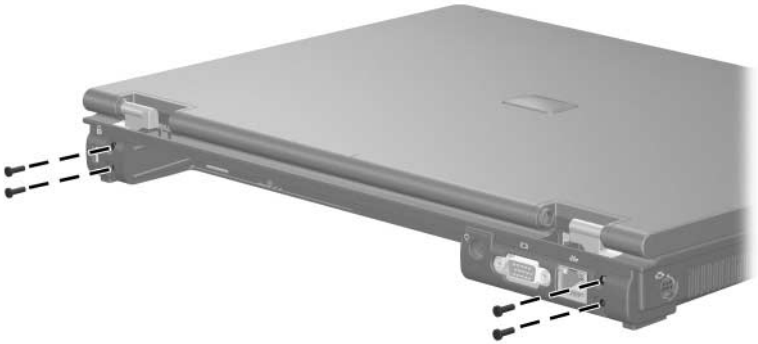
Removing the Display Assembly Screws
