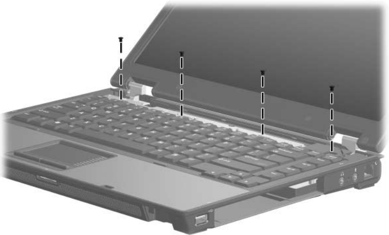
Removing the Keyboard Screws
