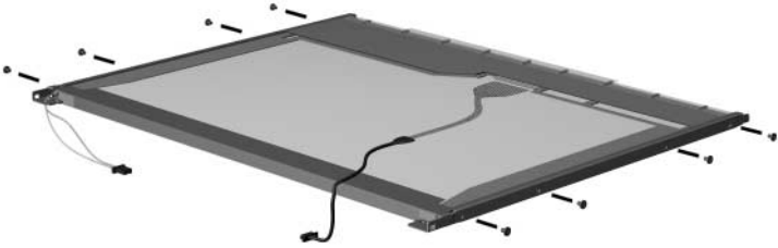
Removing the LCD Panel Frame Screws
