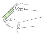
6. Hold the DIMM by the edges, and align the notches on the DIMM with the DIMM slot. (Check that the locks on each side of the DIMM slot are open.)
