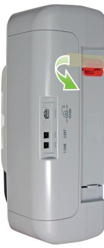
d. Remove the orange plastic insert and tape from the back of the Printing Mailbox.
