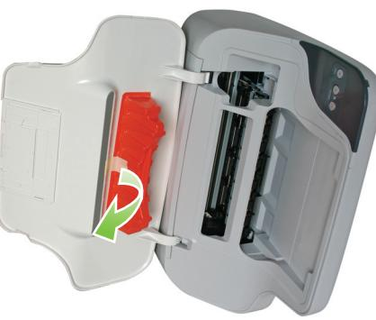
c. Remove the orange plastic insert and tape.
