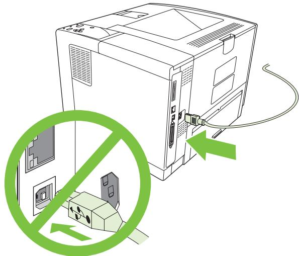
**9.1)** If installing the printer on a network, connect the network cable.
