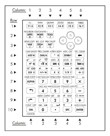
The figure shows 10 rows of keys combined with 3, 5, or 6 columns. Row 1 has 6 keys, rows 2 and 3 have 3 keys each, and rows 4 through 10 have 5 keys each. There are 4 arrow keys located on the right-hand side of the keyboard in the space occupied by rows 2 and 3.
