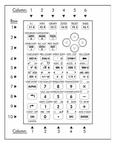
The figure shows 10 rows of keys combined with 3, 5, or 6 columns. Row 1 has 6 keys, rows 2 and 3 have 3 keys each, and rows 4 through 10 have 5 keys each. There are 4 arrow keys located on the right-hand side of the keyboard in the space occupied by rows 2 and 3. Each key has three, four, or
