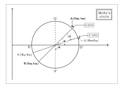
The stress condition for which the shear stress,  $\tau'_{xy'}$  is zero, indicated by segment D'E', produces the so-called *principal stresses*,  $\sigma^P_{xx}$  (at point D') and  $\sigma^P_{yy}$  (at point E'). To obtain the principal stresses you need to rotate the coordinate system x'-y' by an angle  $\phi_n$ , counterclockwise, with respect to the system x-y. In Mohr's circle, the angle between segments AC and D'C measures  $2\phi_n$ .
