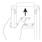
b. Insert 4 new AAA (LRO3) batteries into the main compartment. Make sure each battery is inserted in the indicated direction.
