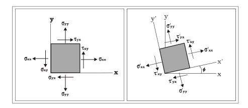
The relationship between the original state of stresses ( $\sigma_{xx}$ ,  $\sigma_{yy}$ ,  $\tau_{xy}$ ,  $\tau_{yx}$ ) and the state of stress when the axes are rotated counterclockwise by f ( $\sigma'_{xx}$ ,  $\sigma'_{yy}$ ,  $\tau'_{xy}$ ,  $\tau'_{yx}$ ), can be represented graphically by the construct shown in the figure below.
