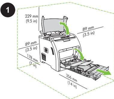
**1** **Prepare the location.** Place the printer on a sturdy, level surface in a well-ventilated area. Make sure that the air vents are not blocked and all doors can open freely.
