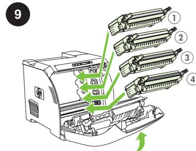
Reinstall the four print cartridges and close the front door.
