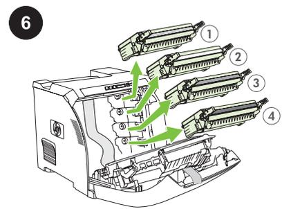
**Remove the FOUR print cartridges by holding the blue handles on both sides of each cartridge and then pulling straight out.**
