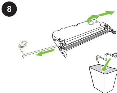
Remove the two shipping locks and pull the tape completely out of the four print cartridges.
