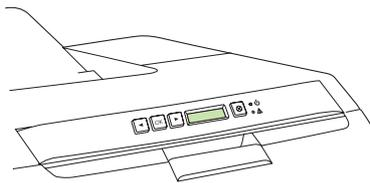
**Set the media size and type for the input trays.** At the control panel, press **OK**, select **SYSTEM SETUP**, and then press **OK**. Select **PAPER SETUP**, press **OK**, and then select media sizes and types for each tray.
