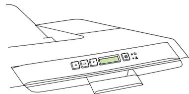
**Configure an IP address, if necessary.** At the printer control panel, press **OK**, press the **<** or **>** buttons to select **Network Config**, and then press **OK**. Press the **<** or **>** buttons to select **TCP/IP Config**, and then press **OK**.
