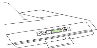
**Find the IP address or the Bonjour printer name by printing a Network Report.** At the control panel, press **OK** to select **Main Menu**, and then press **OK**. Select **Network Report**, and then press **OK**.
