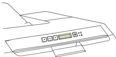
**Find the IP address by printing a Configuration Page.** At the printer control panel, press **OK** to select **Main Menu**, and then press **OK**. Press the **<** or **>** buttons to select **Network Report**, and then press **OK**.
