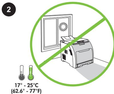
**2** **Regulate the environment.** Do not place the printer in direct sunlight or in an area that has abrupt temperature and humidity changes.
