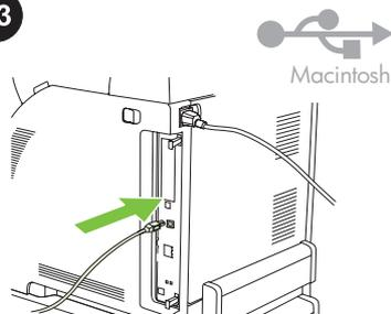
**Connect the USB cable.** Connect a USB cable that is no longer than 2 meters (6.5 feet) to the printer and the computer. Restart the computer. HP does not recommend using USB hubs with this printer.
