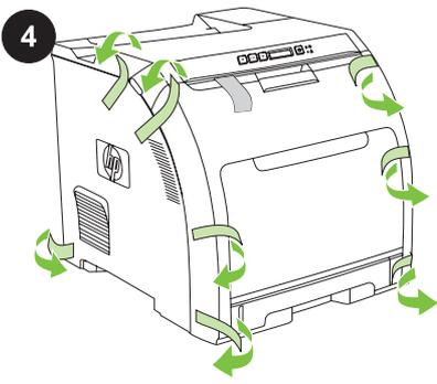
**Remove all shipping tape.** Check the device thoroughly and remove all of the shipping tape.
