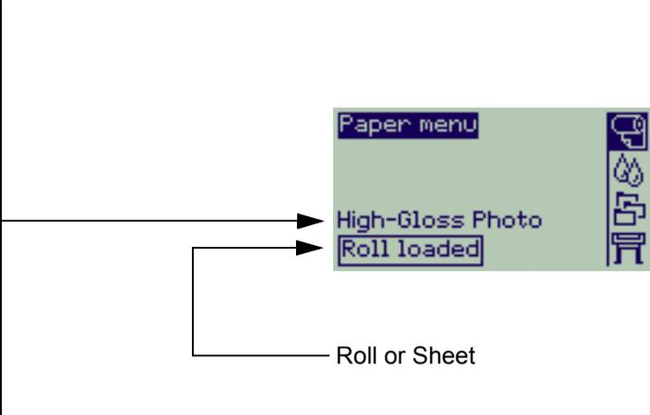
If there is no paper loaded the front panel display shows the following message and you will need to load roll or sheet media.
