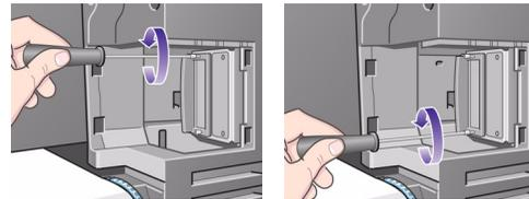
5. When you have inserted the card, screw it into place, using its two screws (at the top and bottom of the card). Again, this can be done with a screwdriver or manually.
