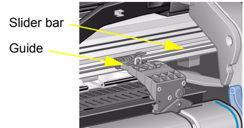
5. If necessary, lift the blue paper lever, to release any trapped paper. Remember to lower it again when you have finished.
