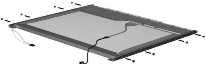
Removing the LCD Panel Frame Screws
