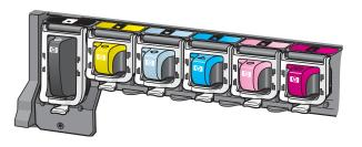
Match the color and pattern of the ink cartridge to the color and pattern on the print carriage.
