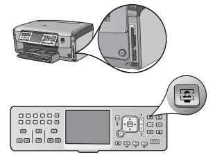
a Insert the memory card from your camera into the appropriate memory card slot and press the **Photosmart** Express button.
