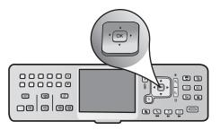
**c** Press the arrow buttons to view the desired photo.
