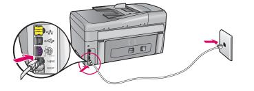
Connect one end of the supplied phone cord to the port labelled **1-LINE** and the other to a wall jack.
