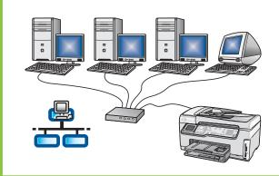
Use this connection type if you want an Ethernet cable connection between the HP All-in-One and your network. Equipment needed: router and Ethernet cable. For an Ethernet cable connection, go to Section B (page 9) for instructions.
