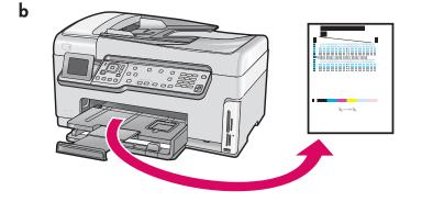
a After you close the access door, a prompt appears to load plain white paper. Make sure paper is loaded, and then press OK to start the process. The device initializes the ink cartridges and aligns the printer. This takes approximately 5 minutes.
