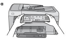
**a** Position the control panel faceplate over the buttons on the device.
