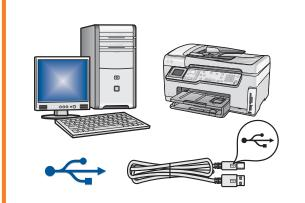
Use this connection type if you want to connect the HP All-in-One directly to one computer. (**Do not connect the USB cable until step A2**).
