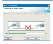
**Problem:** The **Device Setup Has Failed To Complete** screen appears. **Action:** Verify that the control panel faceplate is firmly attached. Unplug the HP All-in-One and plug it in again. Check all connections. Make sure the USB cable is plugged into the computer. Do not plug the USB cable into a keyboard or non-powered hub. Refer to Section A.
