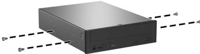
Figure 2-18 Installing Guide Screws in the Optical Drive
