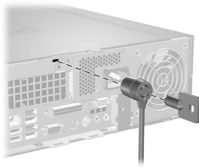
Figure C-1 Installing a Cable Lock
