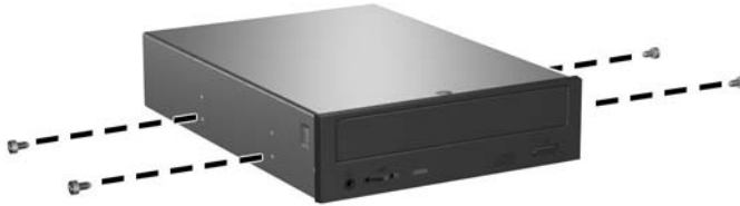
Figure 2-18 Installing Guide Screws (Optical Drive Shown)
