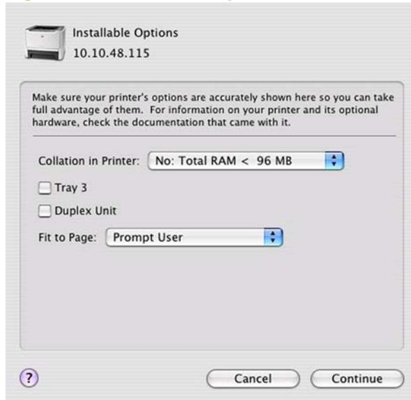
7. In the **Collation in Printer** drop-down menu, select one of the following options, depending on the device configuration:
