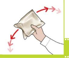
63 After shaking, unwrap each printhead and remove all orange parts.
