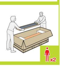
Remove the six box fasteners from the sides of the printer box. To remove a fastener, pull on the tab at the side to open the fastener, then continue pulling to remove the whole thing from the box.
