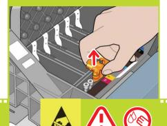
Press the OK key on the front panel when you have removed all of the setup printheads. The front panel then prompts you to install the new printheads.
