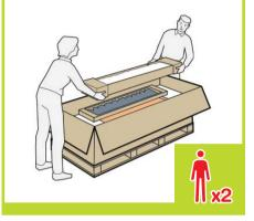
7 Remove the rear tray from the printer.
