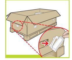
P Lift up the sides and top of the printer box, and remove them from the printer.
