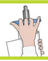
75 Replace the spindle into the printer, left end first, with the fixed stop on the left and the blue removable stop on the right.
