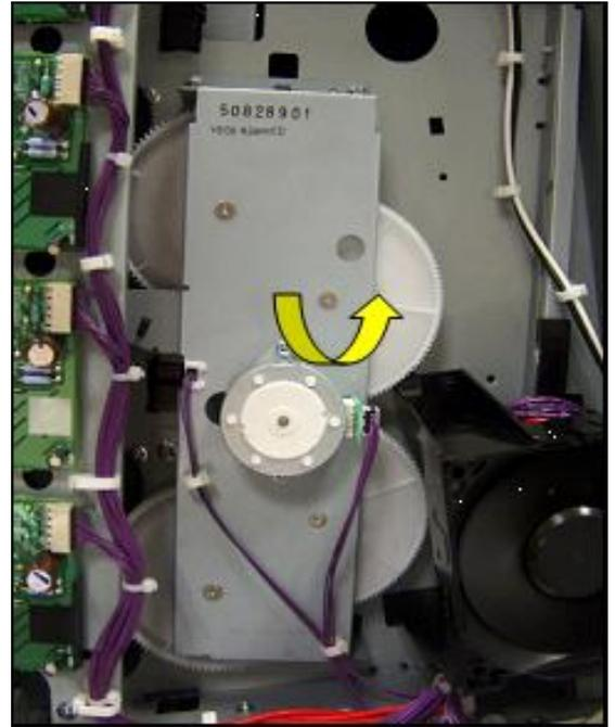
6. When the SCIP cams pop through the sheet metal and are exposed, rotate the SCIP cams on the Developer Alienation Cam towards the front of the printer until the SCIP cams are seated in the “home” position as seen in the second photo on the right (circled yellow).
