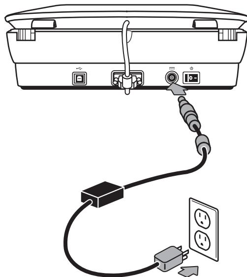
The power supply also has an AC cable that is connected to the power supply on one end and plugged into a power outlet or surge protector on the other end.
