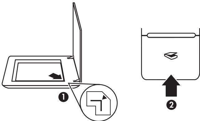
1. Place a photo or document on the scanner glass as indicated by the reference mark on the scanner.
