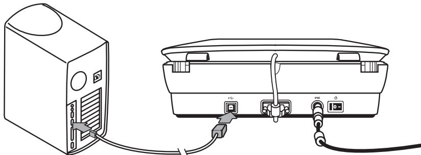
2. Connect the rectangular end of the cable to the computer.
