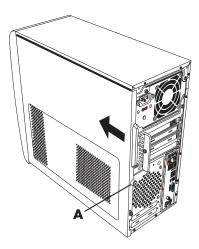
**NOTE:** There is a 3mm gap between the top of the side panel and the top of the chassis when the side panel is attached properly.
