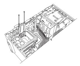
7 Complete the procedures to replace the front panel, replace the side panel, and close the PC. See "Opening and Closing the PC" on page 1.
