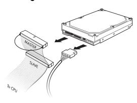
Disconnecting the Parallel ATA hard disk drive cables
