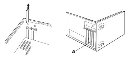
6 If you are not replacing the old add-in card with a new add-in card, close the open slot by inserting the metal slot cover into the opened slot.
