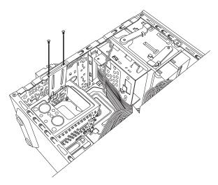
4 Push down the latch on the side of the hard disk drive cage, and then slide the hard disk drive cage away from the bottom of the chassis as shown below.
