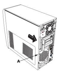
3 Use the handle to pull and slide the panel back about 1 inch (2.5 centimeters), and then lift it off the chassis.
