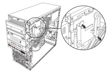
3 Disconnect the power, data, and the sound cable, if available, from the back of the optical drive you want to remove. For most drive cables, use a gentle rocking motion to free the plug. For Serial ATA hard disk drive cables, press the latch (select models only) in the center of each plug, and pull the plug from the drive connector.
