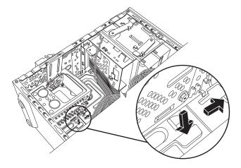
5 Lift the hard disk drive cage out of the chassis, and then remove the hard disk drive cables (1, 2). For most drive cables, use a gentle rocking motion to free the plug. For Serial ATA hard disk drive cables, press the latch (5) (select models only) in the center of each plug (6), and pull the plug from the drive connector.
