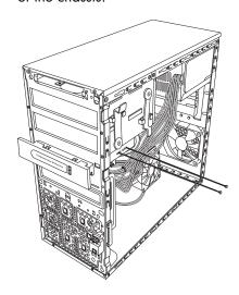
3 Disconnect the power and data cables from the back of the drive by squeezing the two latches and pulling the cable.
