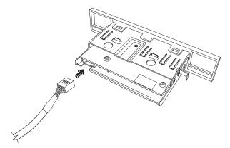
4 Push the memory card reader into the chassis until the screw hole on the chassis is aligned with the screw hole on the right side of the memory card reader, and then insert the screw to secure the memory card reader to the chassis.
