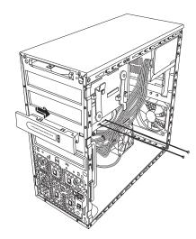
4 Connect the power and data cables to the back of the HP Pocket Media, diskette (floppy), or hard disk drive.
