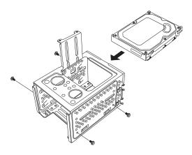
3 Place the hard disk drive cage into the chassis. The two screw holes on the hard disk drive cage (A) should be aligned with the screw holes on the chassis (B).
