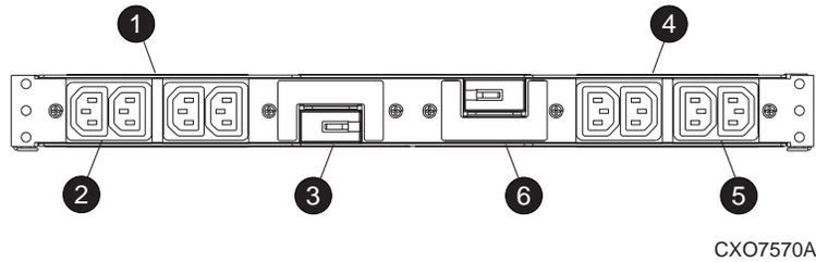
**Figure 66 Dual PDU assembly—top view**
