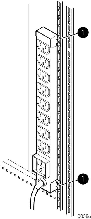
**Figure 70 Rack-mounted 252638-001 PDM**
