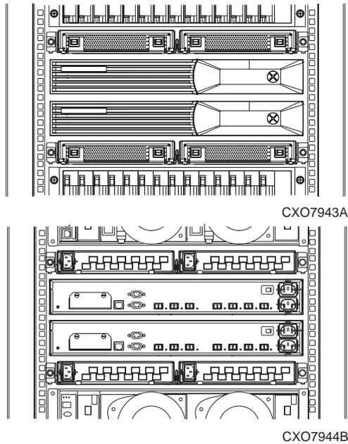
**Figure 7 HSV110 controller location—front and rear views**
