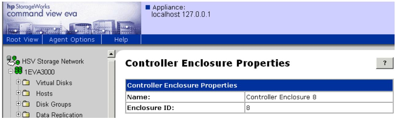
**Figure 35 Controller Enclosure Properties page**
