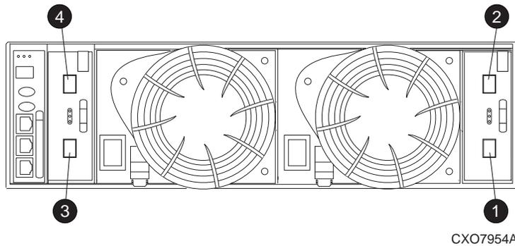
**Figure 79 Transceiver element numbering**
