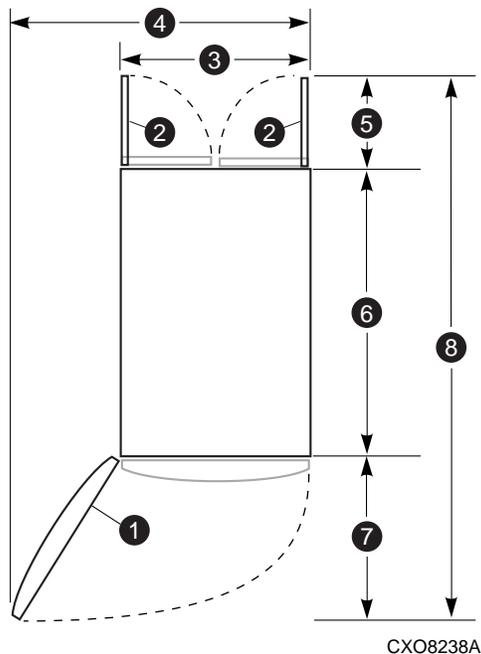
**Figure 72 10000-Series single rack configuration floor space requirements**
