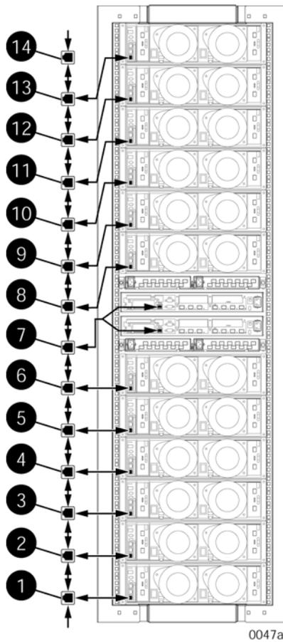
**Figure 55 Enclosure address bus components with shelf ID expansion cables**
