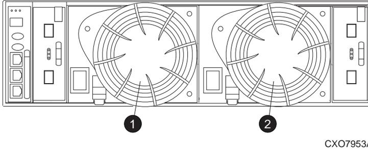
**Figure 77 Blower element numbering**
