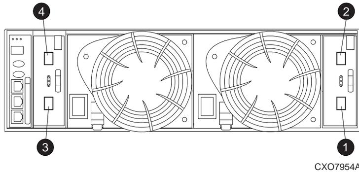
**Figure 40 Input and output ports**
