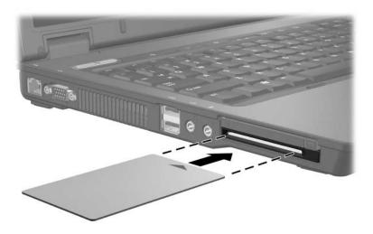
2. Follow the on-screen instructions for logging on to the computer using the smart card PIN.
