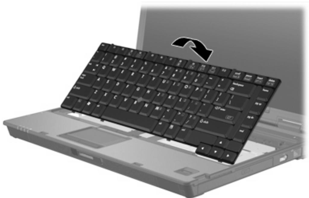
15. Slide the 4 keyboard release latches to lock the keyboard.
