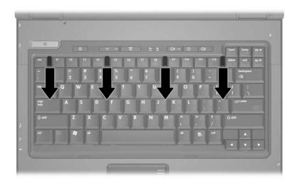
13. Gently lift the top edge of the keyboard and tilt the keyboard over until it rests on the palm rest of the computer.
