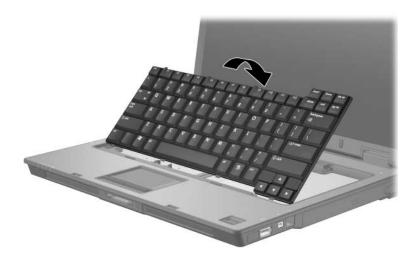
17. Slide the 4 keyboard latches to lock the keyboard.
